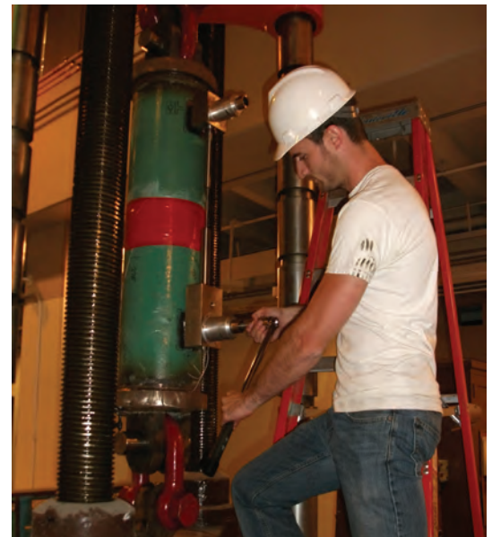
Laboratory performance qualification testing of ROV-serviceable SSSA
