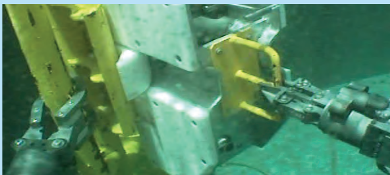
ROV pulling tool away from the sensor during ROV qualification tank testing
