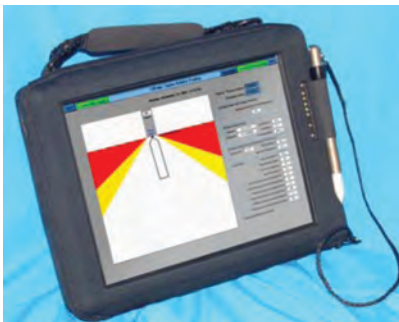
Typical PTU tablet with operator screen display
