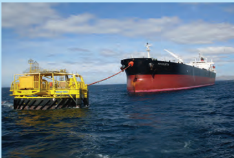
Buoy RTU transmitting Hawser Tension to a moored tanker
