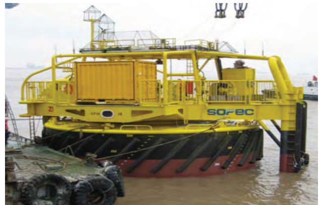
CALM Buoy replacement for the TERMAP facilities in Comodoro Rivadavia
